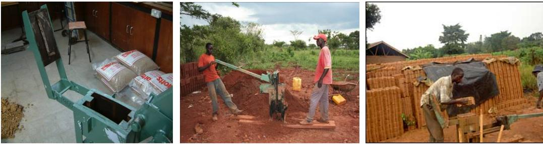
**Figure 1:** Interlocking Stabilised Soil Block (ISSB) using a Makiga Ram
